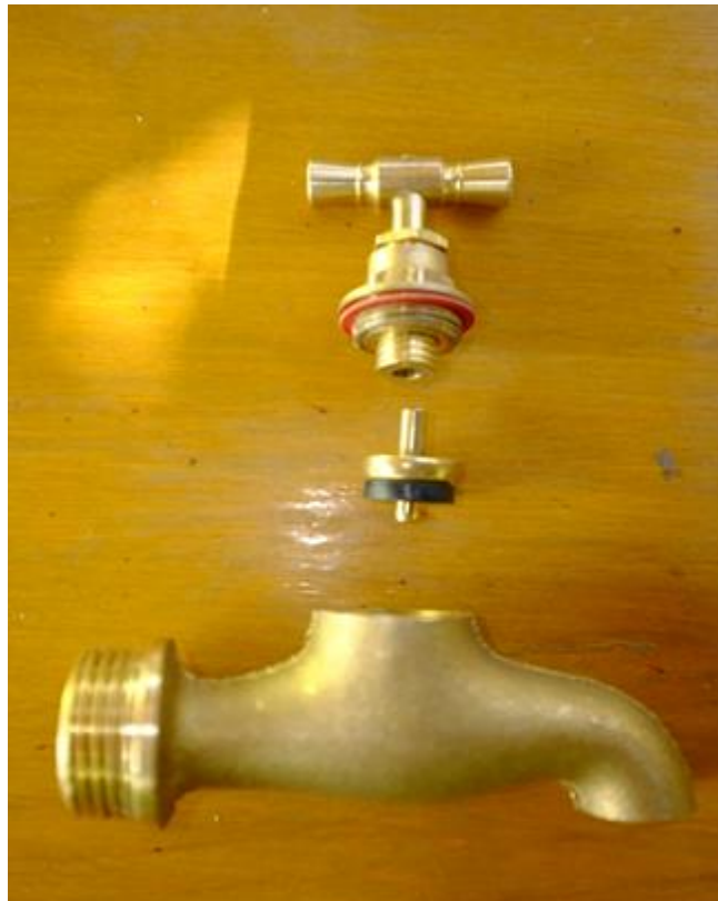
Picture 32: Water tap with replaceable rubber washer
