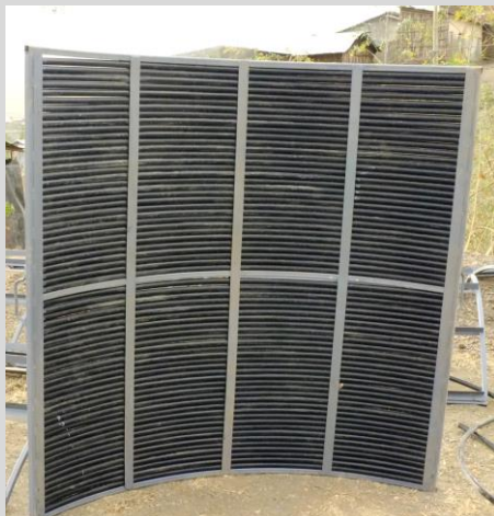
Pictures 5&6: Kalamino cistern body mold; 1/4 circle sections Pictures 5 & 6: The PVC pipes are fixed permanently onto the steel frame of the four body mold circular sections. This makes the mold lighter and easier to handle. The horizontal lining of the PVC pipes provides an ideal cement profile (after inside cement plastering and removal of the mold) for outside cement plastering (see Picture 17).
