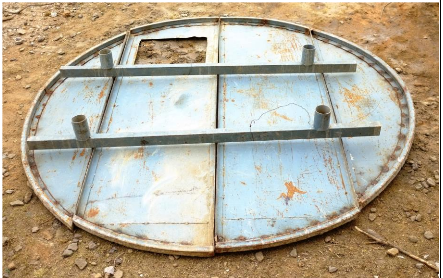
Picture 11: Kalamino cistern cover mold – seen from below
